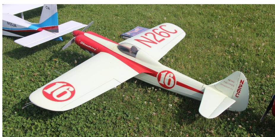
Robert Storick's Shoestring with electric power and 2.4 Ghz for the throttle control
