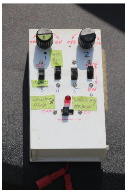
These electronic controls attached to the handle for flaps and throttle
