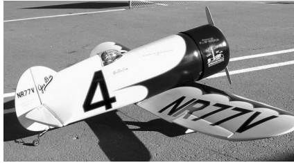
My Gee Bee Z fully fueled, and waiting for the frequency to clear. It placed 2nd in Civilian. It was built from a Jack Devine Models kit, is 30% scale, spans 85", is powered by a Briston 3.2, and weighs 24 pounds.
