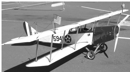
Just a sample of the marvelous aircraft seen at the 1/8th Air Force. This Jenny spans 12.5 feet, and is powered by a G-62.
