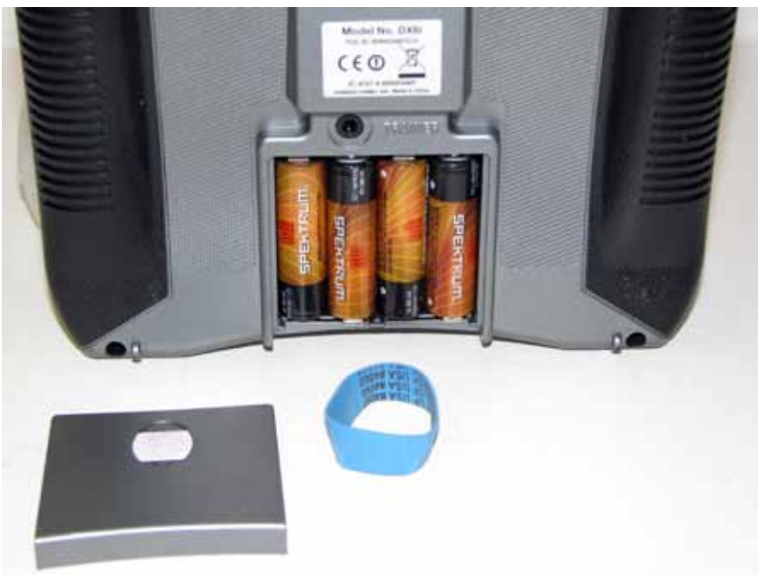
Photo showing the inside of the battery compartment and the connector tabs.
