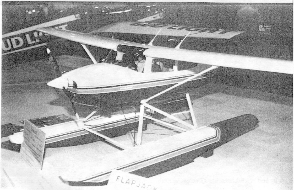
This is the Cessna 182 built by Vince Pettke from a Top Flite kit. 16 lbs. Saito 1.50.
